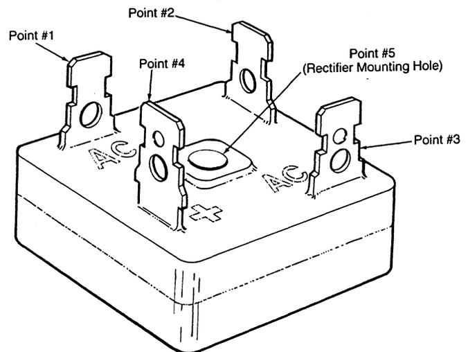
E. Place the positive (+) lead on point #1 and the negative (-) lead on point #3. The Ohmmeter again should not register any deflection (no deflection indicated infinite resistance). Reverse these connections and the Ohmmeter should again register no deflection. IF THE RECTIFIER FAILS ANY OF THE PREVIOUS TESTS (A - E), REPLACE THE RECTIFIER BECAUSE IT IS DEFECTIVE.
