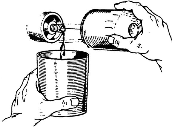
When installing the new oil filter element, wipe the filter gasket's sealing surface on the engine block free of oil and apply a thin coat of clean engine oil to the rubber gasket on the oil filter. Screw the filter onto the threaded oil filter stub, and then tighten the filter firmly by hand.
