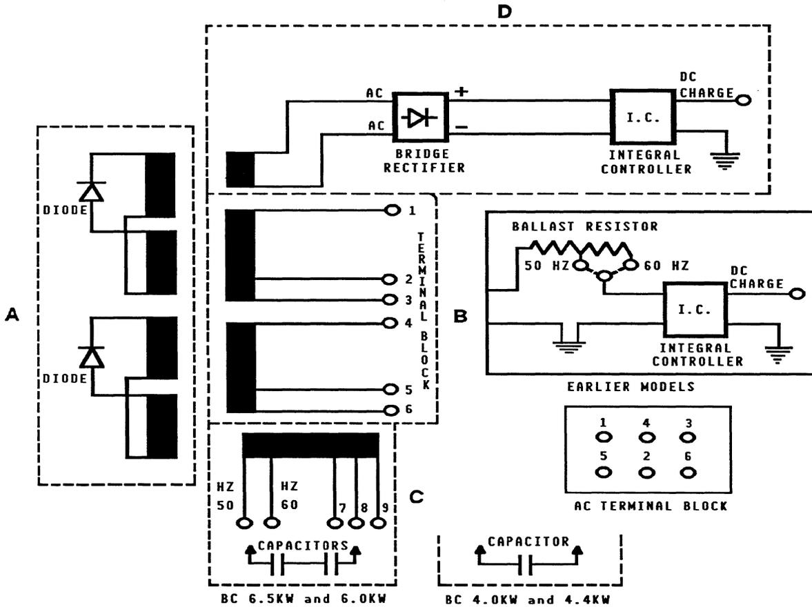
Generator Internal Wiring Schematic with
