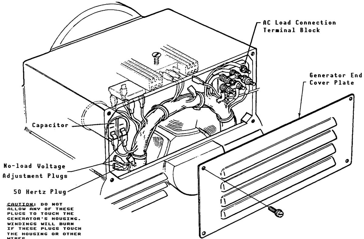
**CAUTION: DO NOT ALLOW ANY OF THESE PLUGS TO TOUCH THE GENERATOR'S HOUSING. WINDINGS WILL BURN IF THESE PLUGS TOUCH THE HOUSING OR OTHER WIRES.**
