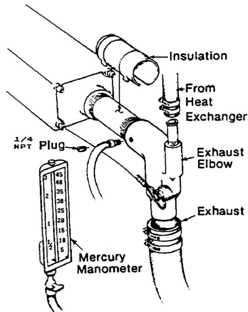
A water column can be made by taking a clear plastic tube and taping one end of the tube along a yardstick and fitting the other end of the tube with a 1/4 inch NPT (National Pipe Tap) pipe fitting.
