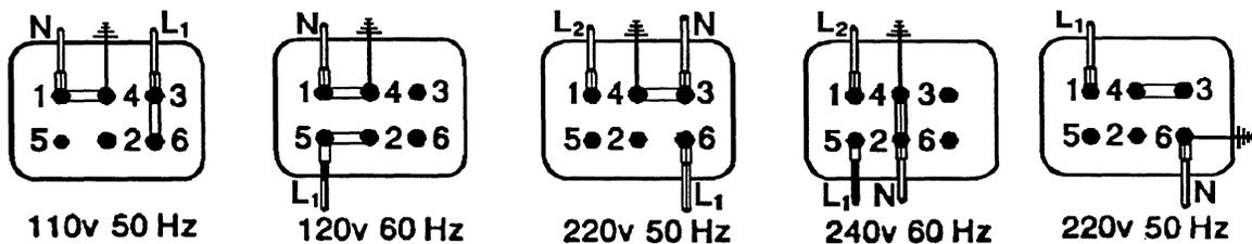
4. Shut off the generator. Make sure the correct Hertz lead (60 Hertz #6, or 50 Hertz #5) is plugged into the capacitor. Refer to the illustration on the top of the next page.
