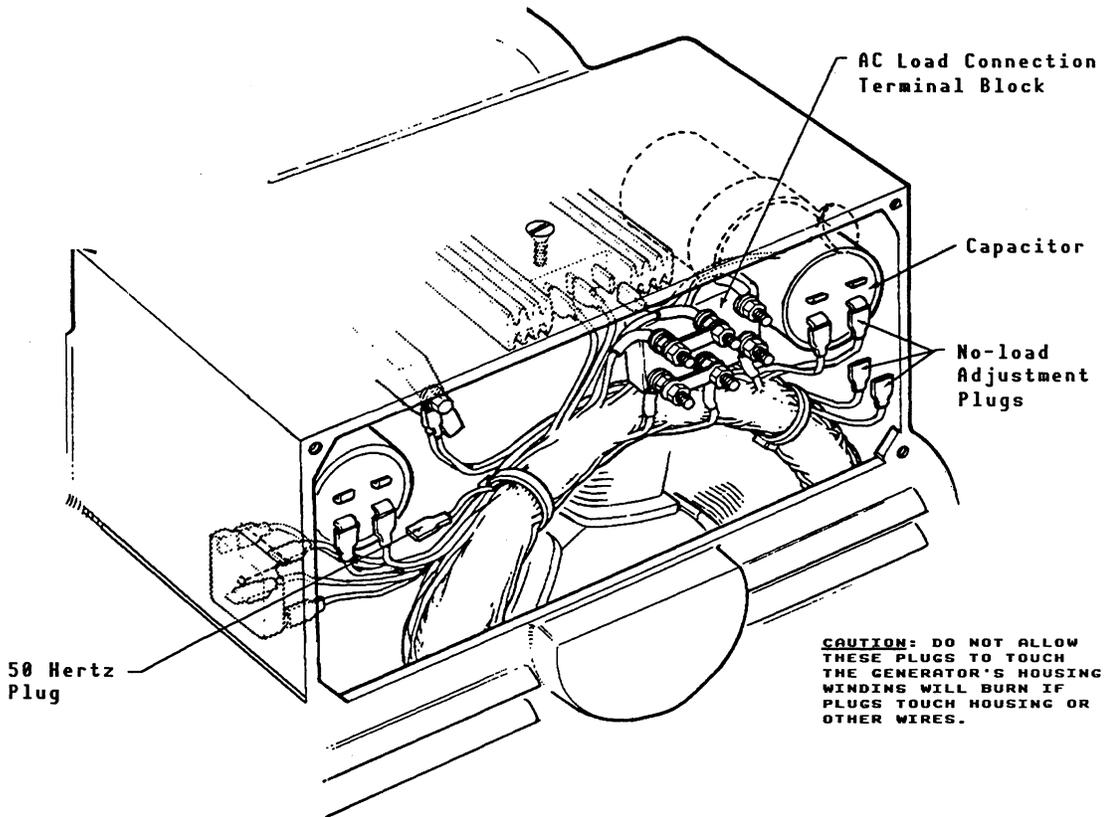
**CAUTION:** DO NOT ALLOW THESE PLUGS TO TOUCH THE GENERATOR'S HOUSING. WINDINGS WILL BURN IF PLUGS TOUCH HOUSING OR OTHER WIRES.
