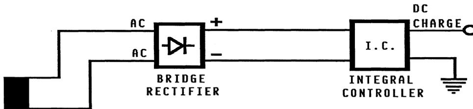
Normal DC voltage running out of the rectifier (in Volts DC) is measured across the two DC connections of the bridge rectifier; that is, + and -.
